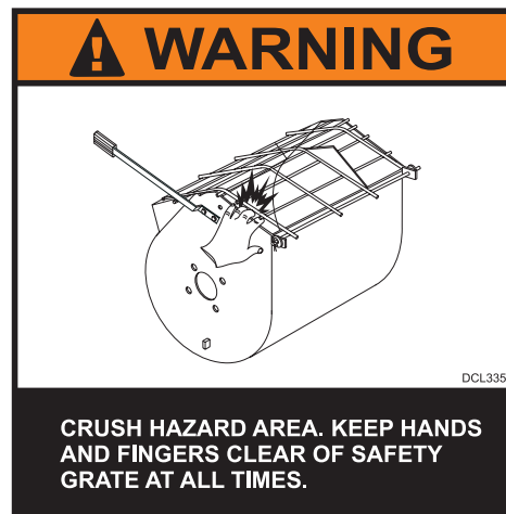
Figure 38. Safety Grate (Crush Hazard)
